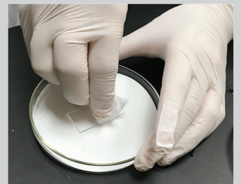
Wipe glass surface • Allow treated surface to remain undisturbed for the given contact time • The surface is not assessed for wetness
